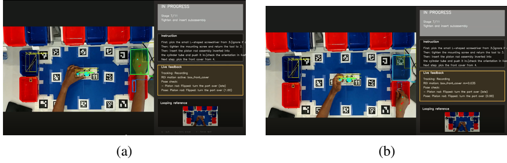
Figure 9.4: (a) The ROI has a strong border and prominent color fill indicating Active, (b) ROI has only a visible boundary indicating no Active and signaling user to pick component from that box
