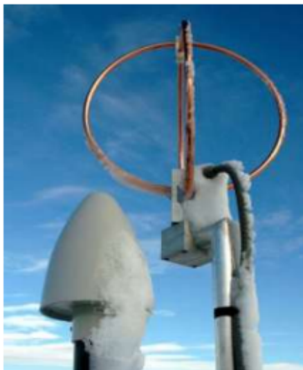
Figure 2.4: Antenna of a LINET sensor and GPS. Source: Reproduced from Petracca [28].
