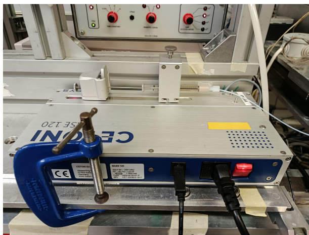
Figure 2.10: Photo of the remotely controlled pump syringe
