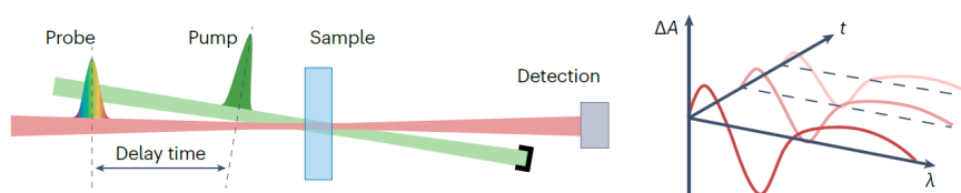
Figure 1.1: Schematic representation of a pump & probe transient absorption experiment (adapted from [1]). In the left image there is a schematic representation of a pump signal exciting the sample and the probe signal monitoring the system’s evolution after delay time \Delta t . In the right one the difference absorbance spectrum ( \Delta A ) induced by the pump is sketched for different delay times t
