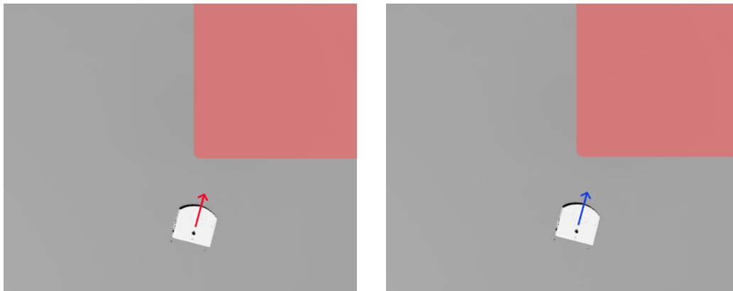
Figure 3.9: Behavior of the robot before reaching an area with dangerous temperatures. The red vector representing the robot control policy and the blue vector representing the resulting vector are the same.
