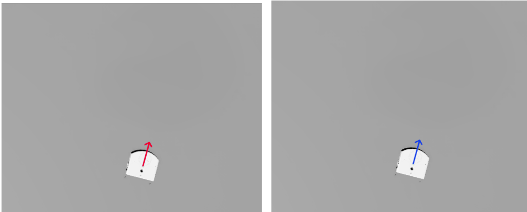
Figure 3.7: Behavior of the robot when it is going forward at maximum speed for a duration that does not pose a danger for the motors. The red vector representing the robot control policy and the blue vector representing the resulting vector are the same.
