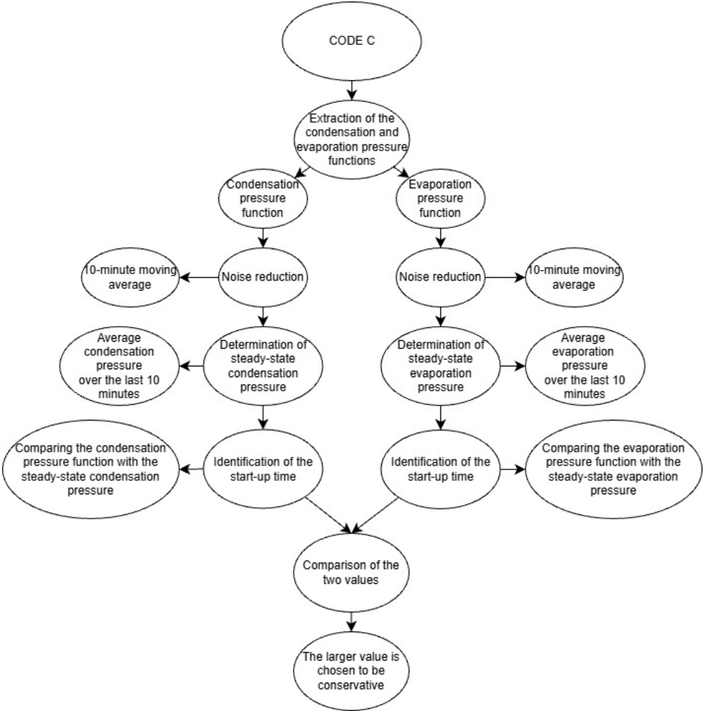
Figure 2.13 - Schematic representation of the MATLAB code C for the thermal start-up time determination
