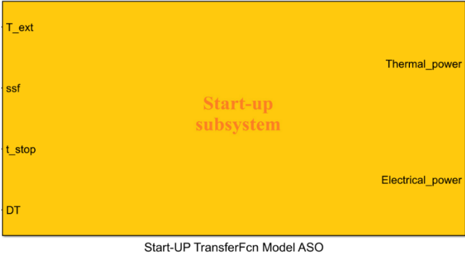
Figure 3.12 - Interface of the transfer function model for ASO with inputs on the left and outputs on the right
