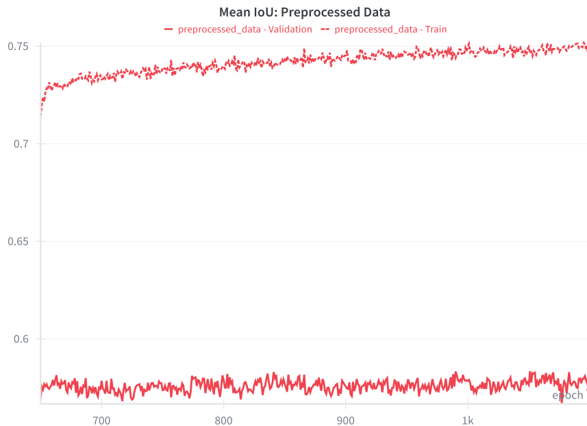
Figure 4.14: Mean training and validation IoU computed over the five folds of the cross validation for the HSSN framework.
