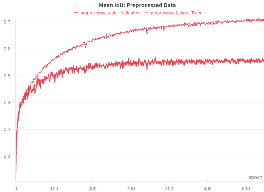
Figure 4.12: Mean training and validation IoU computed over the five folds of the cross validation for the HSSN framework.
