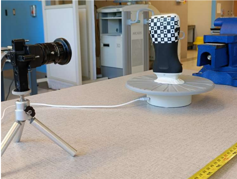
Figure 5.38: 6×10 HydraMarker attached to Clarius L7 ultrasound probe.
