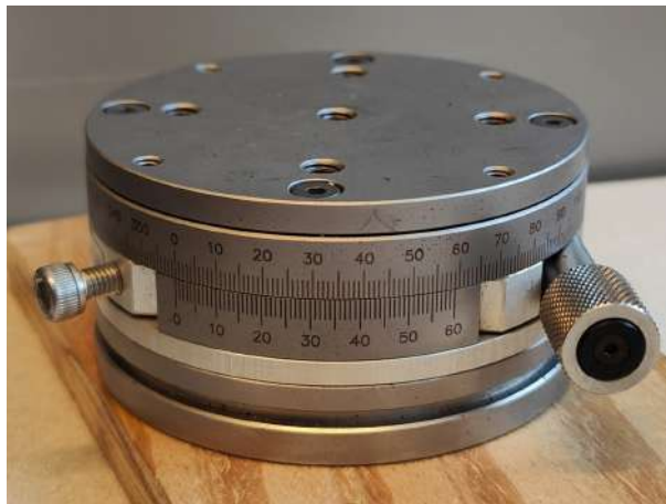
Figure 4.1: Rotational stage (Newport M-UTR80) used for ground truth angular displacements.
