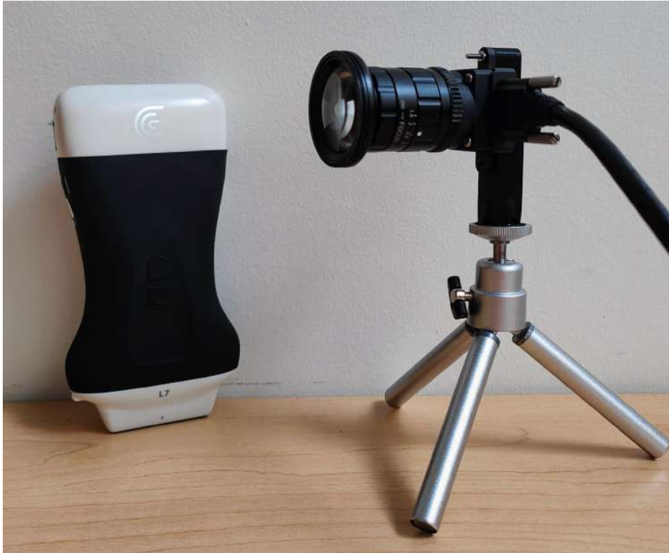
Figure 3.1: 2D Ultrasound Clarius L7 probe (left). Basler daA1920-160uc and Edmund Optics Lens assembly (right).
