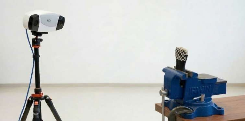
Figure 5.40: Digitization setup with the NDI Polaris Vega (left) and the Clarius probe clamped on the rig.
