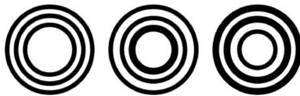
Figure 2.6: CCTag marker examples with three crowns. Each marker is uniquely identified by the crown thickness, encoding a marker ID. Image from the CCTag documentation, used with permission (MPL 2.0) (Calvet et al. 2016).
