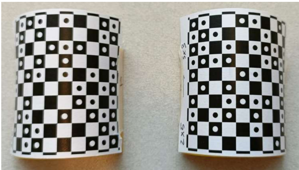
Figure 5.34: Marker A (left) and Marker B (right): two 10 \times 10 HydraMarker fields with 3 \times 3 and 2 \times 5 ID tags, mounted on cylindrical surfaces.
