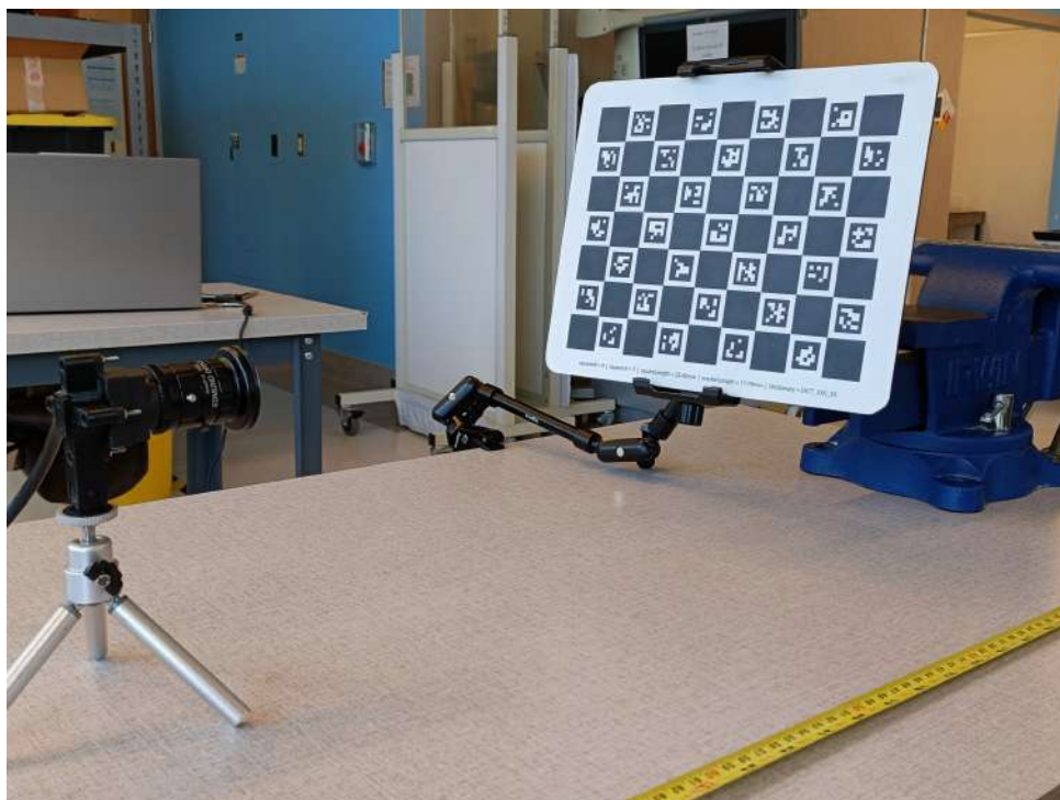
Figure 4.3: Calibration setup showing the ChArUco board positioned at the working distance for intrinsic parameter and distortion coefficient estimation.
