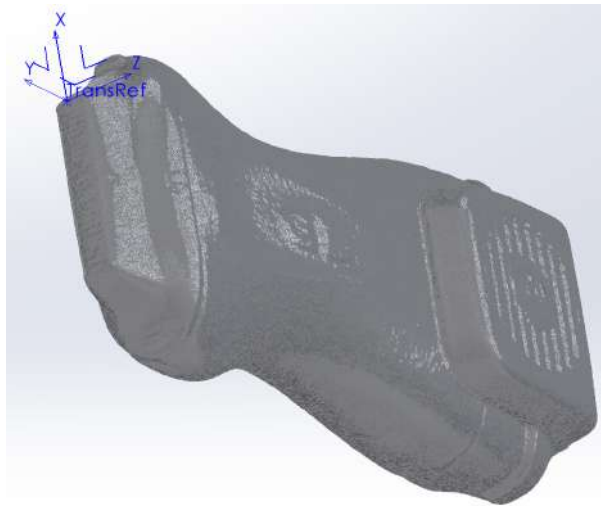
Figure 3.6: 3D model of the Clarius probe with the coordinate frame located on the transducer with MFA orientation.
