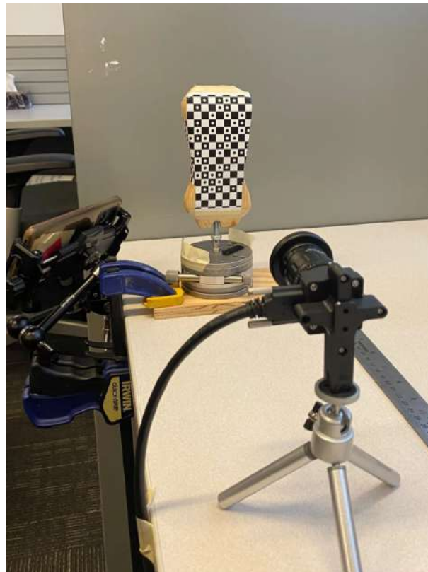
Figure 5.4: 15 \times 17 HydraMarker with 4 \times 4 , and 2 \times 8 ID tags mounted on the probe prototype for rotation testing around the beam axis.
