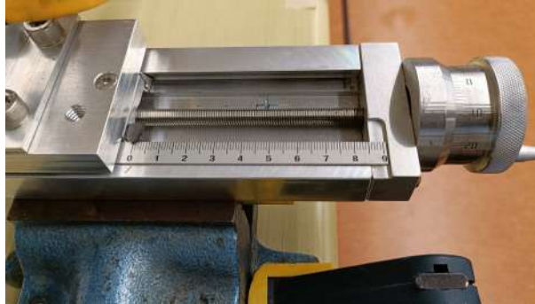
Figure 4.2: Translational stage (Velmex UniSlide® A25 Series) used for ground truth linear displacements.
