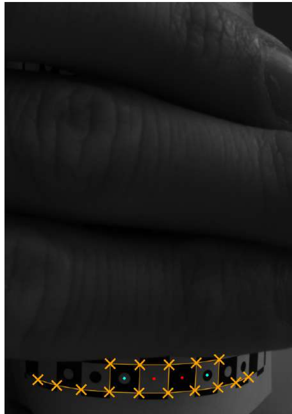
Figure 5.33: Occlusion robustness of the HydraMarker: example frames (a–g) showing progressive hand occlusion with successful corner detection and identification across varying visible marker extents.
