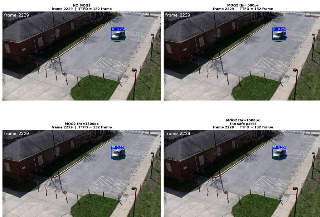
Figure 5.2: Threshold ablation – YOLO11-S INT8. All four configurations produce the same detection frame (frame 2229, TTFD = 132), confirming that the model is the binding constraint regardless of gate settings. Ground-truth boxes in green, predicted boxes in blue.
