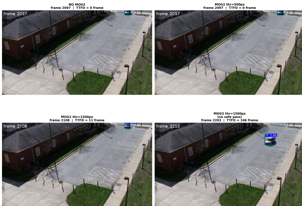
Figure 5.1: Threshold ablation – YOLO11-M FP16. First valid detection frame for each configuration (top-left: NO_MOG2, TTFD = 0; top-right: MOG2_500, TTFD = 0; bottom-left: MOG2_1500, TTFD = 11; bottom-right: MOG2_1500 without safe-pass, TTFD = 106). Ground-truth boxes in green, predicted boxes in blue.
