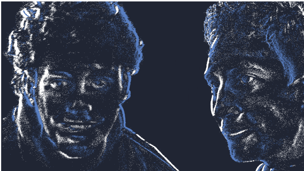
Figure 4.15: Visualization of raw event data (accumulation window) processed via Metavision Studio.
