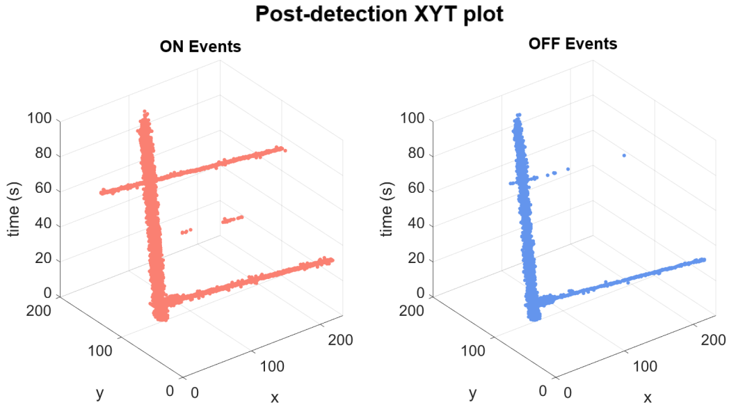
Figure 3.9: Processed event stream derived from the SL-8 R/B recording, following the application of feature detection algorithms and noise filtering of the events.
