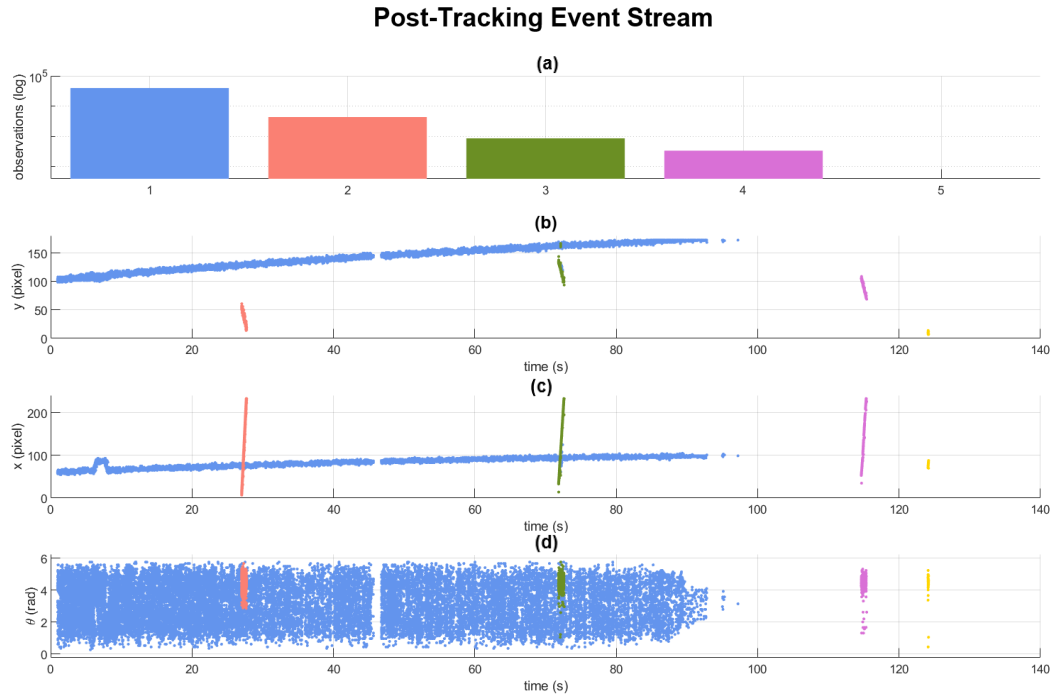
Figure 3.10: (a) Number of tracking events per object; panels (b) and (c) show the tracker event position in x and y respectively over time, while (d) shows the angular direction.
