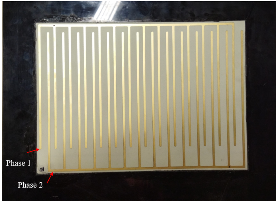
Figure 5.2: View of the exposed electrodes of the DBD actuator used during the tests. The black frame around the actuator is the mask used to block it inside the test section door.
