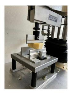
Figura 17- Three point bending test.
