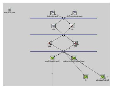
Figura 28 - FederatorBroker, modulo OMNeT++
