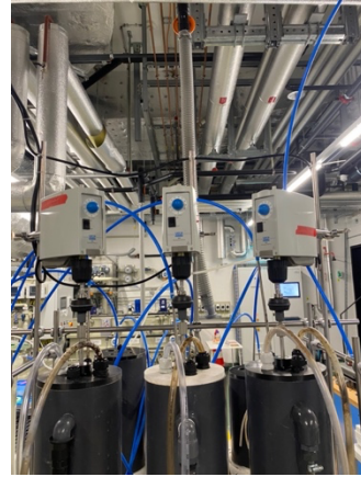
Figure 6: stirrers on sludge reactor Type 1
