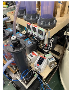
Figure 11: autosampler dosing system + diclofenac dosing system (Ismatec ICC)
