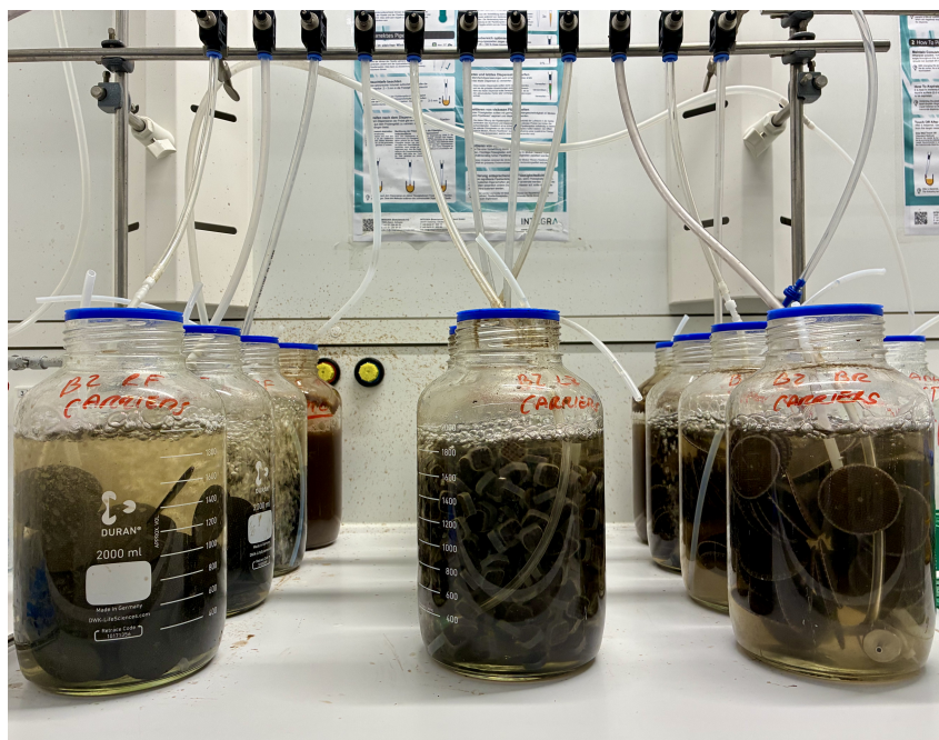
Figure 2.4.2: Batch test setup for diclofenac removal experiments. In the picture Carriers from full-scale plants were used: from left to right, Roderstorf, Lenzburg, and Bad Ragaz.
