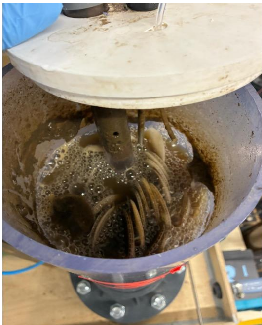
Figure C.0.1: Overview of operational issues encountered in the pilot plant: a) Stop of the main pump before start-up; b) Temporary shutdown of the main plant causing pH drop; c) Clogs and stuck carriers in the MBBR and sludge; d) Floating sludge accumulation in the clarifiers.
