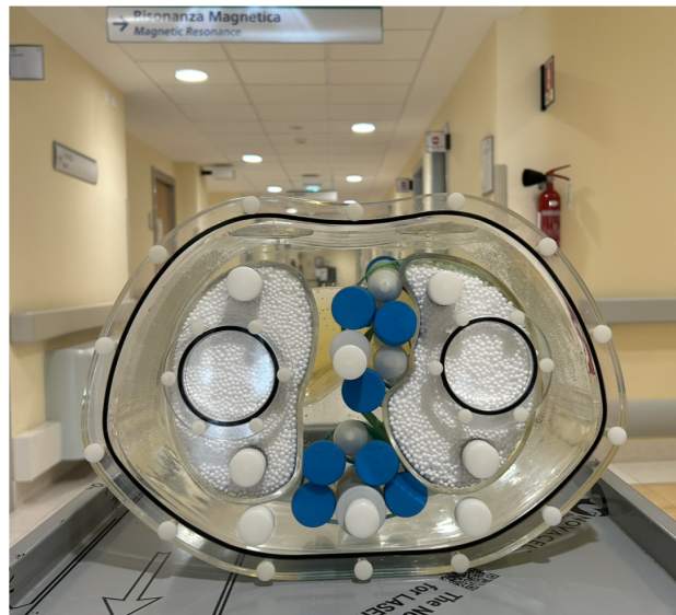
Figure 3.2: Final configuration of the fat-water phantom.
