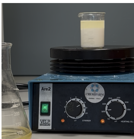
Figure 3.1: Preparation of the fat–water emulsion.
