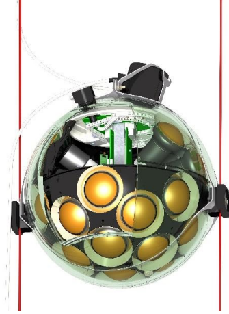
Figure 2.2: Rendering of a KM3NeT DOM with bollards attached to mechanically supporting cables in the deep-sea. In the cut out, the interior of the module with PMTs and electronics is visible [10].
