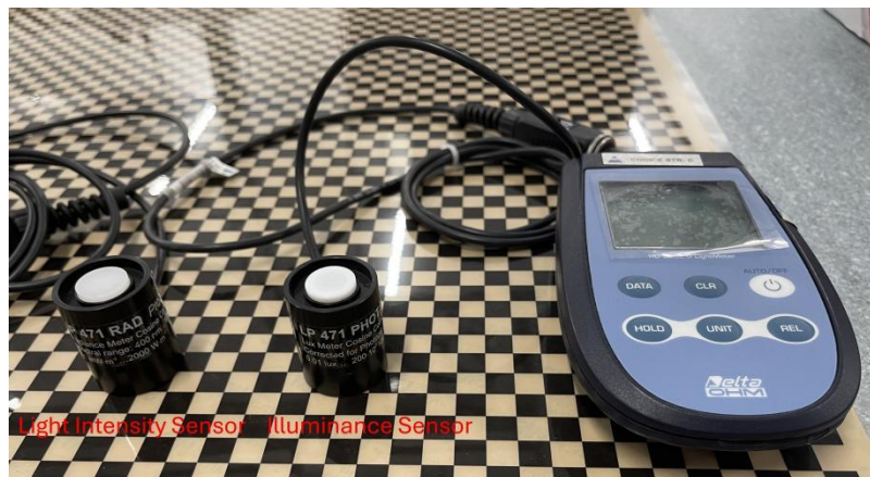
Figure 6. The Reading Tool with Illuminance and Light Intensity Sensors
