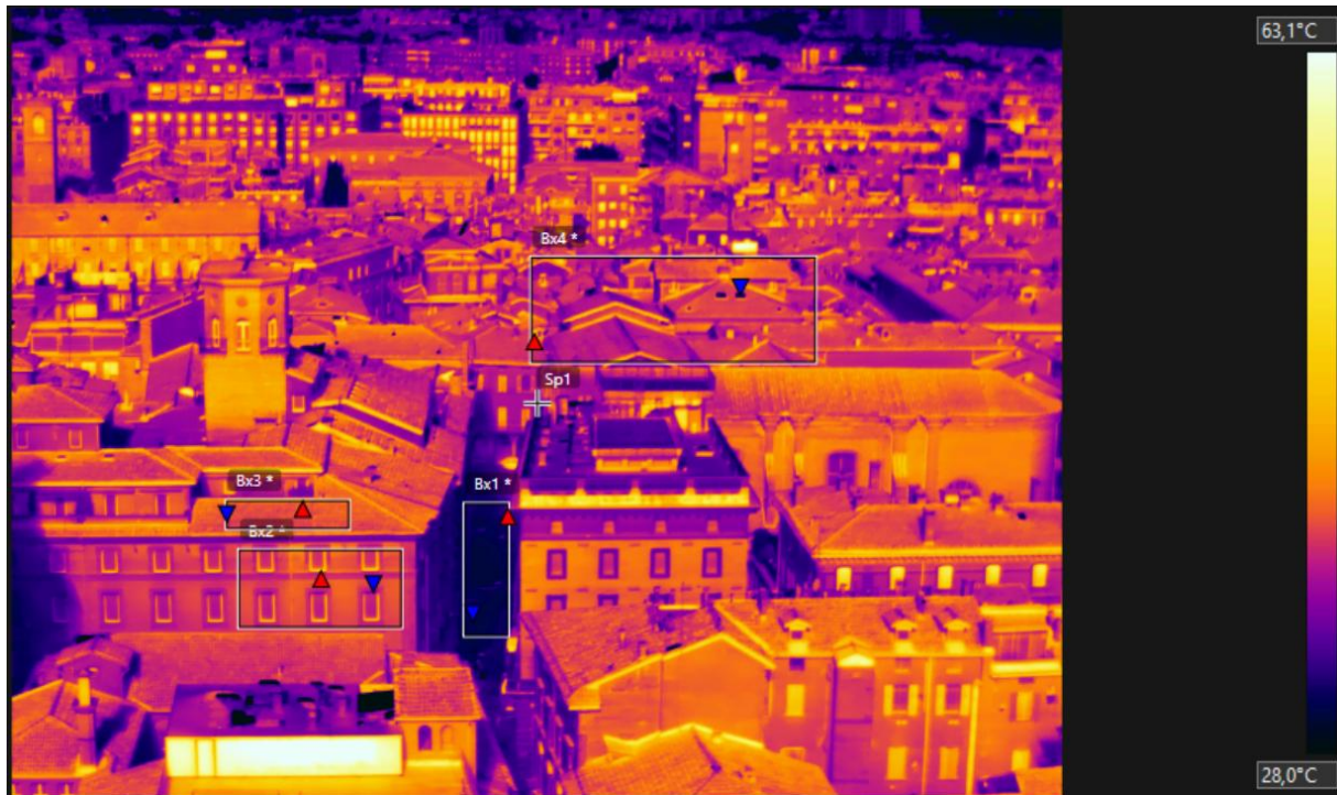
Figure 17 Example of a selection in FLIR Tools: Bx1 was chosen as the reference for a E-W street, Bx2 is an east-facing façade, Bx3 is an east-facing roof, Bx4 is the reference for the east-facing 'roof mix'. This photo was taken at 09:00 CEST, the temperature range is on the right.
