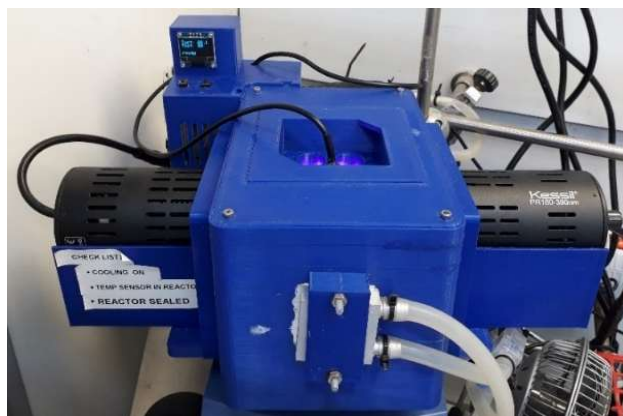
Figure 5.1. Reaction set-up using a temperature-controlled 3D-printed photoreactor under irradiation at 390 nm by two Kessil lamps.
