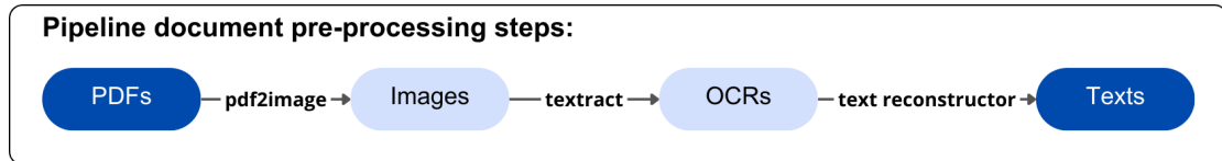
Figure 3.7: The Figure shows the pre-processing schema of a document, from an input PDF to the contained text. illustrates all the steps and techniques used: the pdf2image library, the Textract AWS OCR, and a text reconstructor tool.
