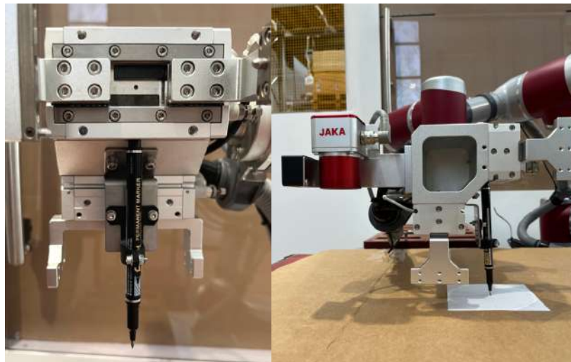
Figure 102 - On the left, the stand attached to the tool. On the right, the drawing operation.
