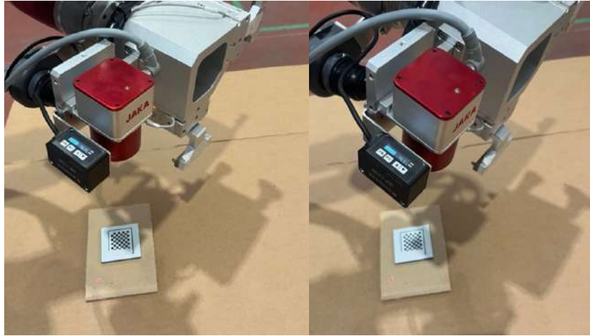
Figure 69 - Representation of two consecutive calibration position.
