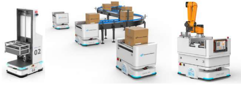
Figure 21 – Different expansion modules for Oasis 600UL. From the left, the forklift module, the conveyor module for material transferring and a robotic arm for object manipulation.
