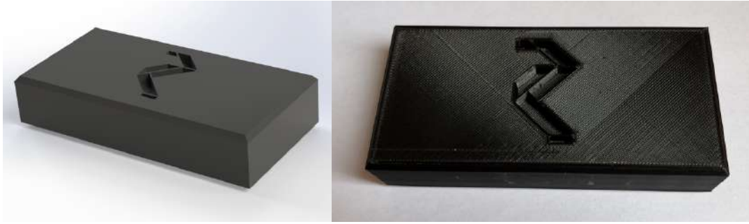
Figure 107 - On the left, the 3D representation of the block, while on the right its realization.
