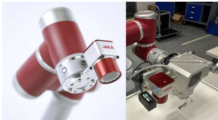
Figure 36 - On the left, the mounting layout suggested from the manufacturer. On the right, the actual position of the camera on the robot gripper.
