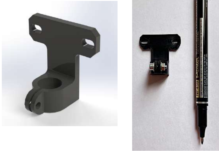
Figure 101 - On the left, the 3D representation of the support. On the right, the support realized with for the proper marker.
