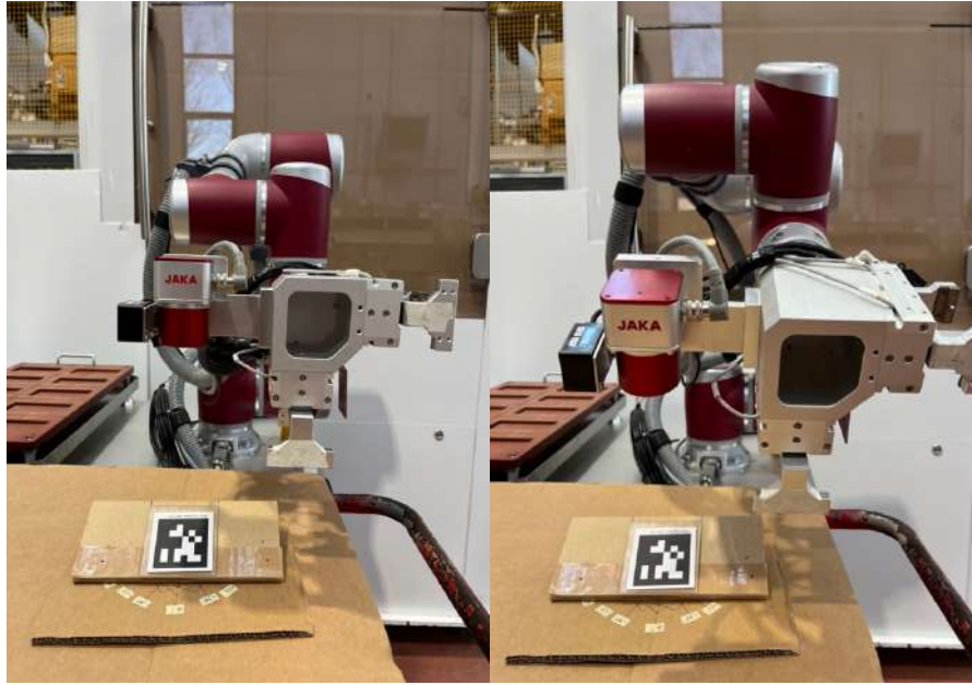
Figure 90 - CASE RX 30°. On the left, the robot in ShootPosition. On the right, the aligned pose of the robot.
