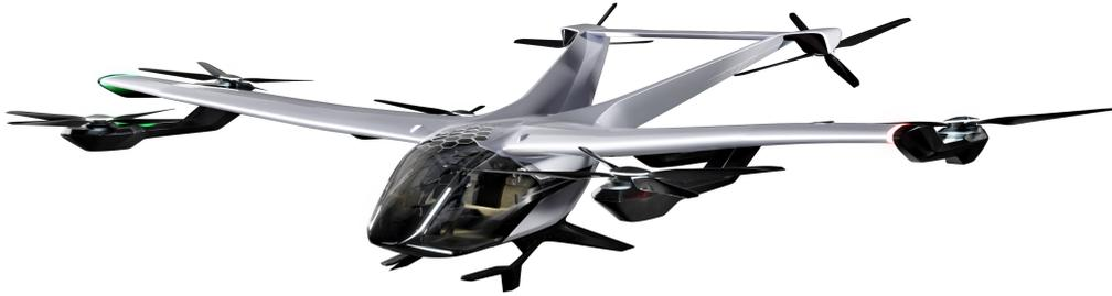
**Figure 1.2:** Compound eVTOL from Airbus: CityAirbus NextGen.<sup>46</sup>
