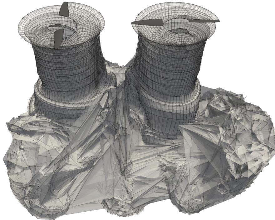
**Figure 4.6:** Snapshot of the developed wake from the two side by side counter-rotating rotors with phase shift  $\Delta\Psi = 90^\circ$ , at the last time step. Left hand rotor stands on the left. Rotor blades are colored in dark grey. The grid lines delimit wake panels, which are slightly transparent to show the internal shape of the wake. We note the asymmetry of the far wake, which is skewed towards the right rotor, causing increased inflow and a smaller average thrust.
