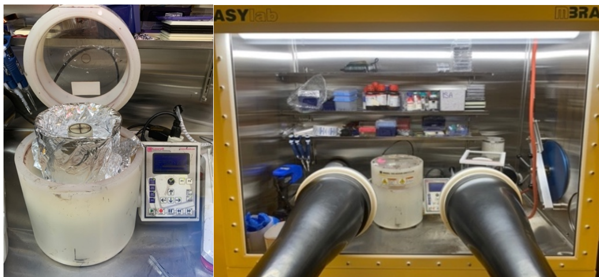
Figure 12 – View of the glovebox and spin coater details.
