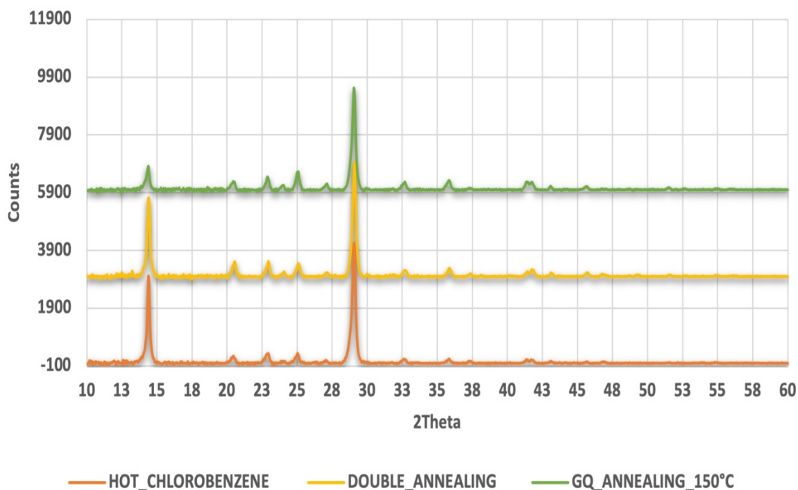
Chart 5 - XRD results for film CsSnI 3 samples. Film 2C (bottom), Film 3C (middle), Film 4C (top). 2-Theta scanning angles from 10° to 60°
