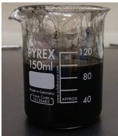
Figure 21: \text{Co}_3\text{O}_4 catalytic ink.
