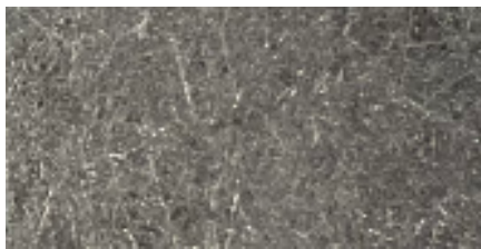
Figure 33: Untreated Ni felt support.
