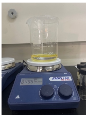
Figure 27: AEM in 3M NaCl solution at 50°C.
