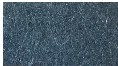
Figure 34: 350°C-treated Ni felt support.
