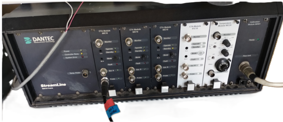
Figure 4.5: StreamLine 90N10 with CTA modules 90C10.
