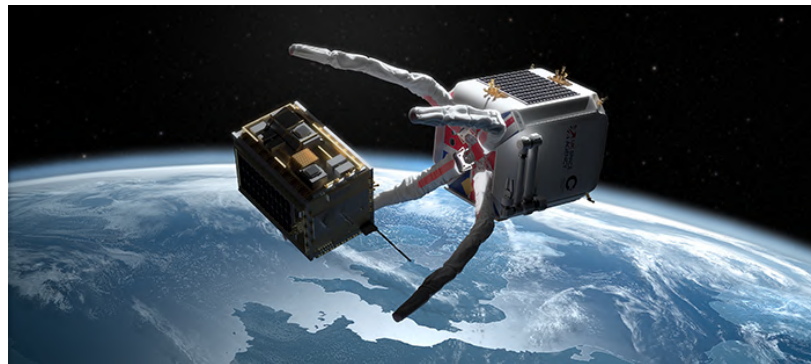
Figure 1.2: ClearSpace spacecraft deorbiting a satellite. Image credit
