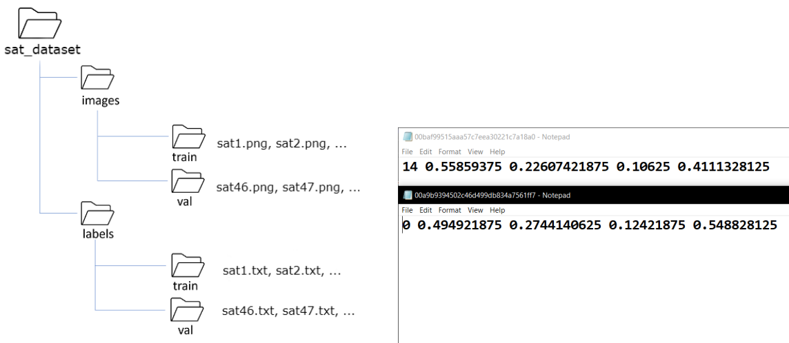
Figure 4.3: Data structure for YOLO.
