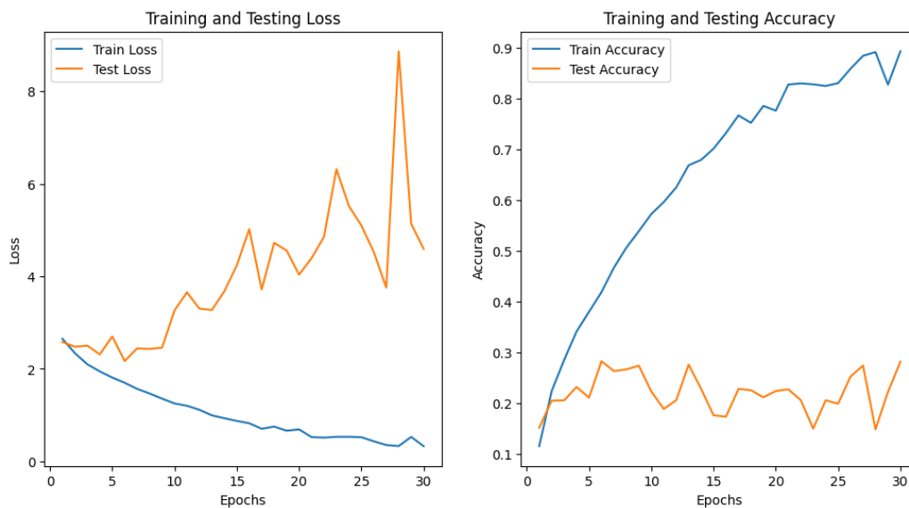
Figure 5.3: Training results over 30 epochs using only image classification.
