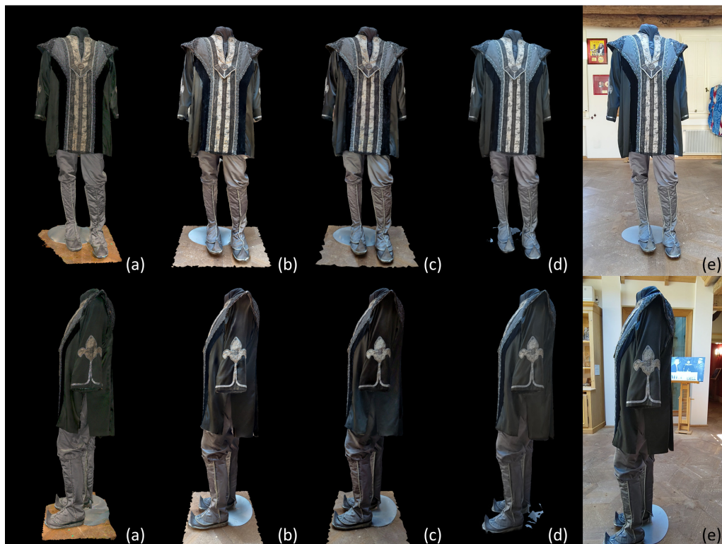
Figure 3.2: Reconstructed model from two different views: front (top row) and side (bottom row). The images are rendered from the resulting mesh reconstruction of a Pavarotti theatrical outfit depicted in (e). The different techniques reported for visual comparison are: (a) Artec Eva (b) Scaniverse (c) Polycam (d) Gaussian Splatting.
