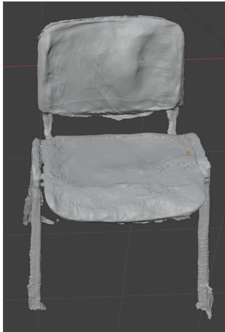
Figure 4.8: Reconstructed mesh using 2DGS technique applying segmentation masking and depth enhanced optimization. The mesh is extracted from the 7000 step snapshot without any further manual processing. The geometry of the object is reconstructed with accuracy even in holes and thin structures. The texture of the surface still presents some artifacts and imperfections.
