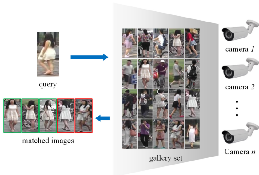
Figure 1.1: [48] The Person Re-Identification task: the query image of a woman is matched against the gallery set produced by n independent cameras. The output is the gallery subset that matches the query identity.
