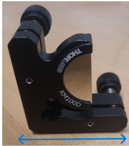
Figure 4.7: Photo of the D-shaped mirror employed as the sample to estimate the idler beam size. The blue arrow indicates the x -direction for the B-scan.
