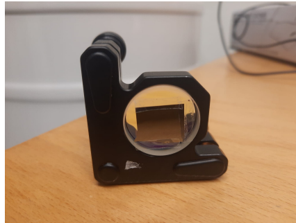
Figure 4.5: Photo of the cut Si layer, carefully attached to the flat \text{SiO}_2 window for measurement.
