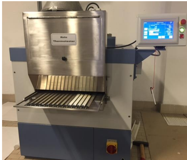
Figure 6.9: Thermotester used to assess colour retention over time
