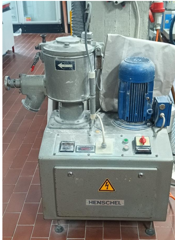
Figure 6.2: lab-scale turbo mixer device form Henschel
