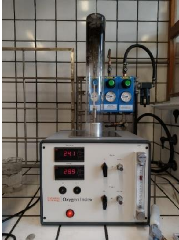
Figure 6.10: equipment used to obtain LOI values.
