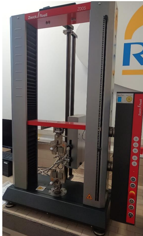
Figure 6.4: Z005 Zwick/Roell dynamometer
