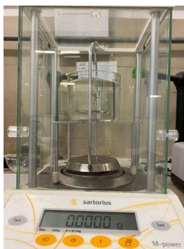
Figure 6.7: instrument used to evaluate relative density
