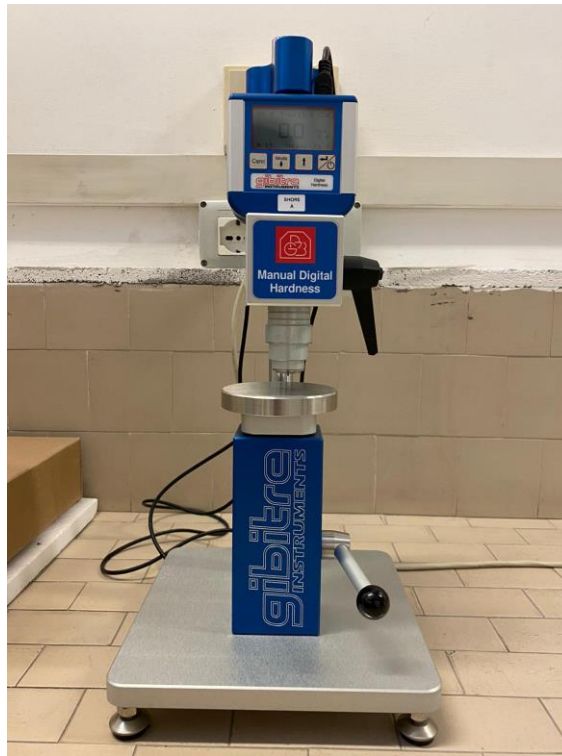
Figure 6.3: manual digital hardness tester from Gibitre Instrument
