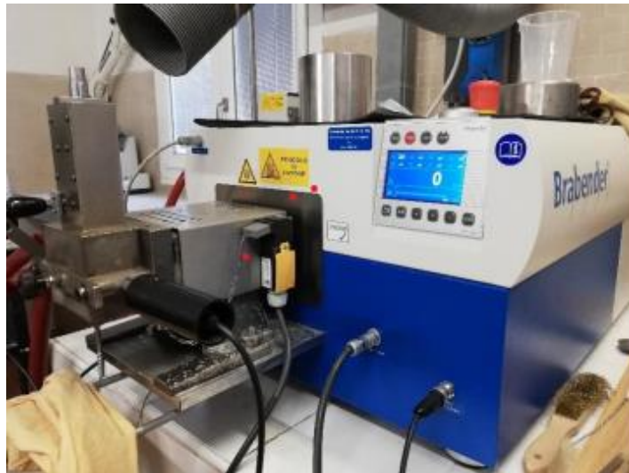
Figure 6.5: plasticorder device from Brabender
