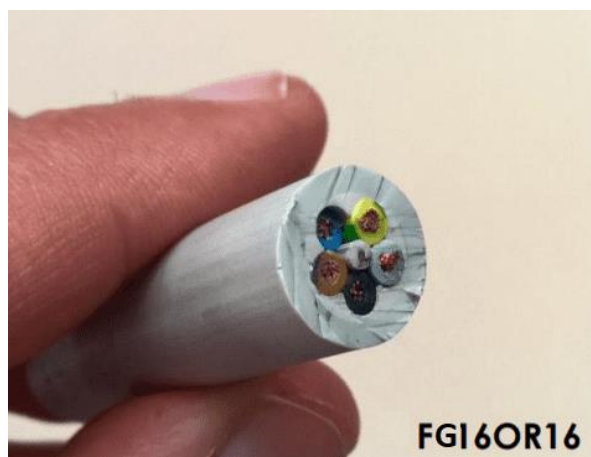
Figure 3.1: FG16OR16 G5X1.5 0.6/1.0 kV Italian electrical cable a.t. CEI UNEL 35016. [35]
