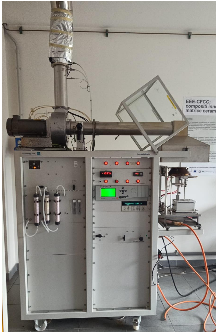
Figure 6.14: cone calorimetry set-up
