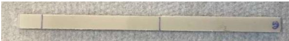
Figure 6.11: specimen of dimensions defined by ASTM D 2863
