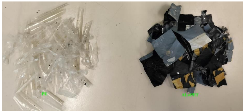
Figure 7 The Delaminated materials.
