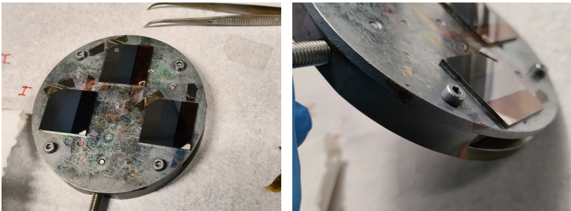
Figure 3.1: On the top: schematics of the sputtering sequence of the sample. The material represented by each color is indicated in the legend. Bottom-left: samples placed on the sputtering sample holder. Bottom-right: close-up of the analyzed sample
