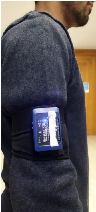
Figure 59: SensorTile.Box PRO kit mounted on the right arm
