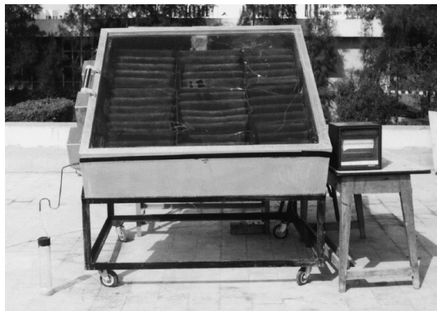
Fig 7 [14] – Experimental apparatus for SAWH (Mansoura University, Egypt)
