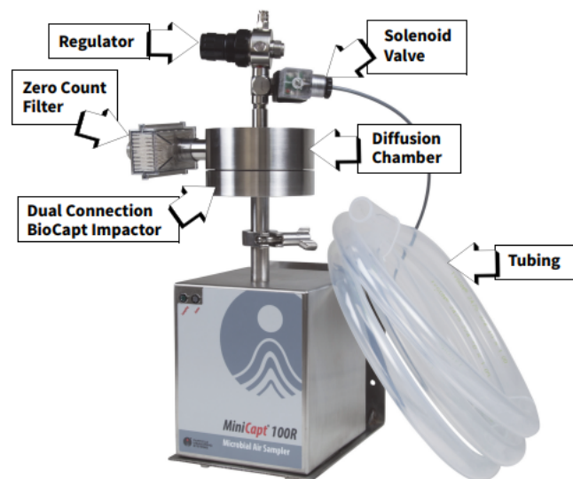
Figure 3.2: MiniCapt 100R Microbial Air Sampler with BioCapt Impactor sampling.
