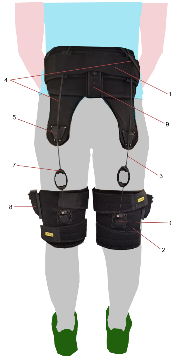
Figure 2.3: Hip exosuit for off-board test. The labels refer to: 1) Elastic belt; 2) Thigh wraps; 3) Cable tendons; 4) Guides to connect the exosuit to the motor device; 5) Upper anchor points; 6) Thigh anchor points; 7) Plastic rings for compliance purposes; 8) Thigh IMUs; 9) Back IMU.
