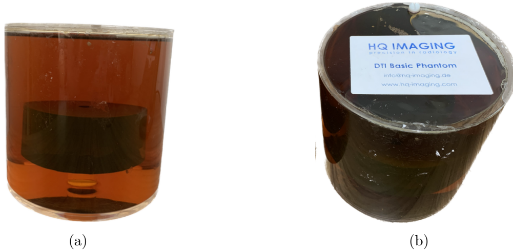
Figure 3.1: (a) Picture of the basic phantom that shows the part in which the fibre bundle is contained and the liquid in which it is immersed. (b) Top vision of the DTI basic phantom with a single fibre ring mimicking restricted anisotropic diffusion.
