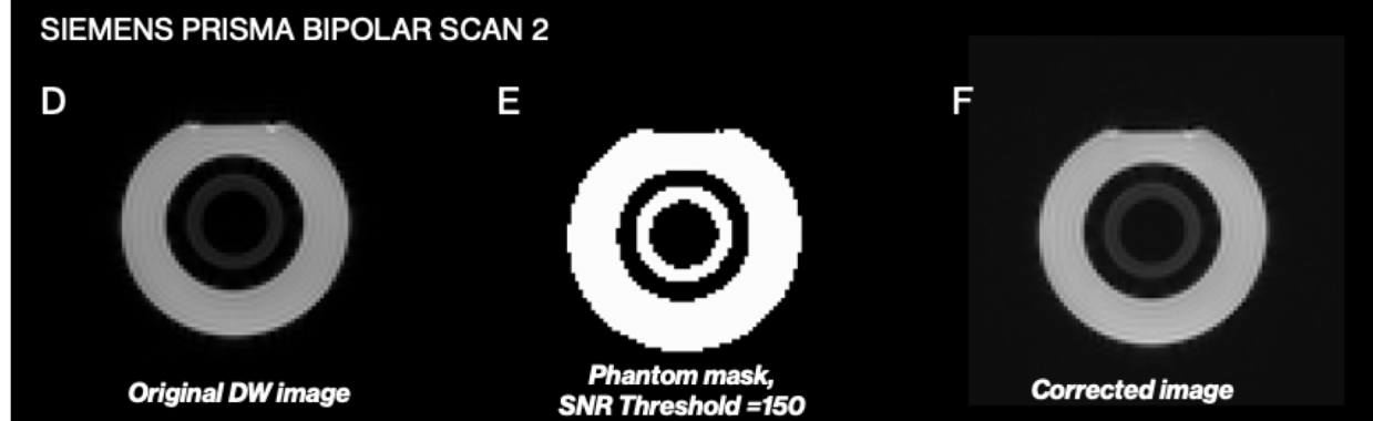
Figure 6.8: Phantom multi-shell Bipolar scan 1 and scan 2 on 3T Siemens Prisma: (A) and (D) Image of the original diffusion-weighted image of the basic phantom, in which it appears to be warped, notably along the phase-encoding gradient direction, (B) and (F) the binary mask constructed using an \text{SNR} = 150 , as displayed, (C) and (E) The corrected DW-image.
