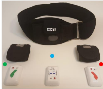
Figure 17 Set of three IMU sensors and belts were utilized during the clinical monitoring. The green and red dots represent the sensors placed on the shoes using Velcro straps, while the light blue dot represents the sensor placed on the lower back using the elastic belt.
