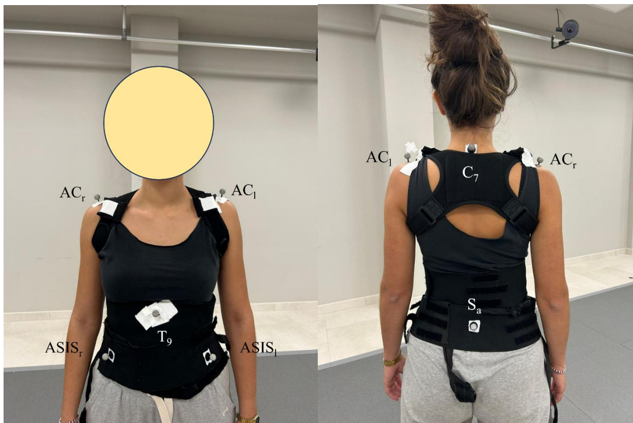
Figure 50 Position of the 7 markers in the correspesctive positions.
