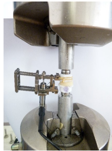
FIGURE 2.10: System without Rekrea anchored mounted on the testing machine.
