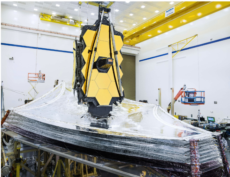
Figure 2.1: JWST in the Northrop Grumman cleanroom following a sunshield deployment test, from G23.
