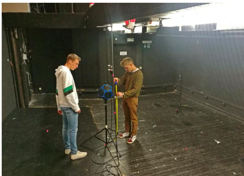
Figure 3.11: Omnidirectional source placement
