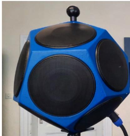
Figure 3.3: Omnidirectional sound source
