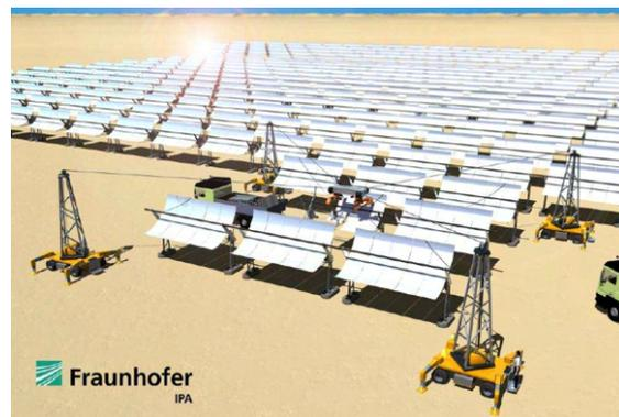
(b) Cable robot for solar panels installation
