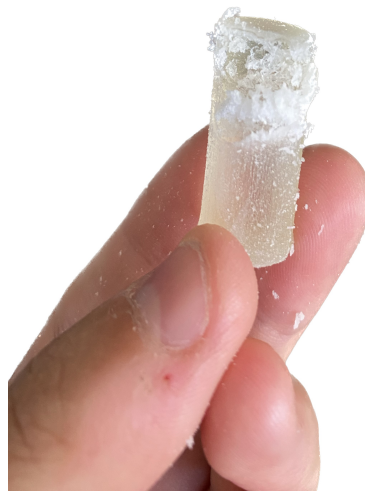
(b) Fracture mode of the HC samples after confined compression test.
