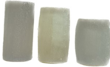
Figure 3.9: Specimens after the mechanical test. From the left, first one is Vero Clear, second one is General Bone and third one Vertebra.
