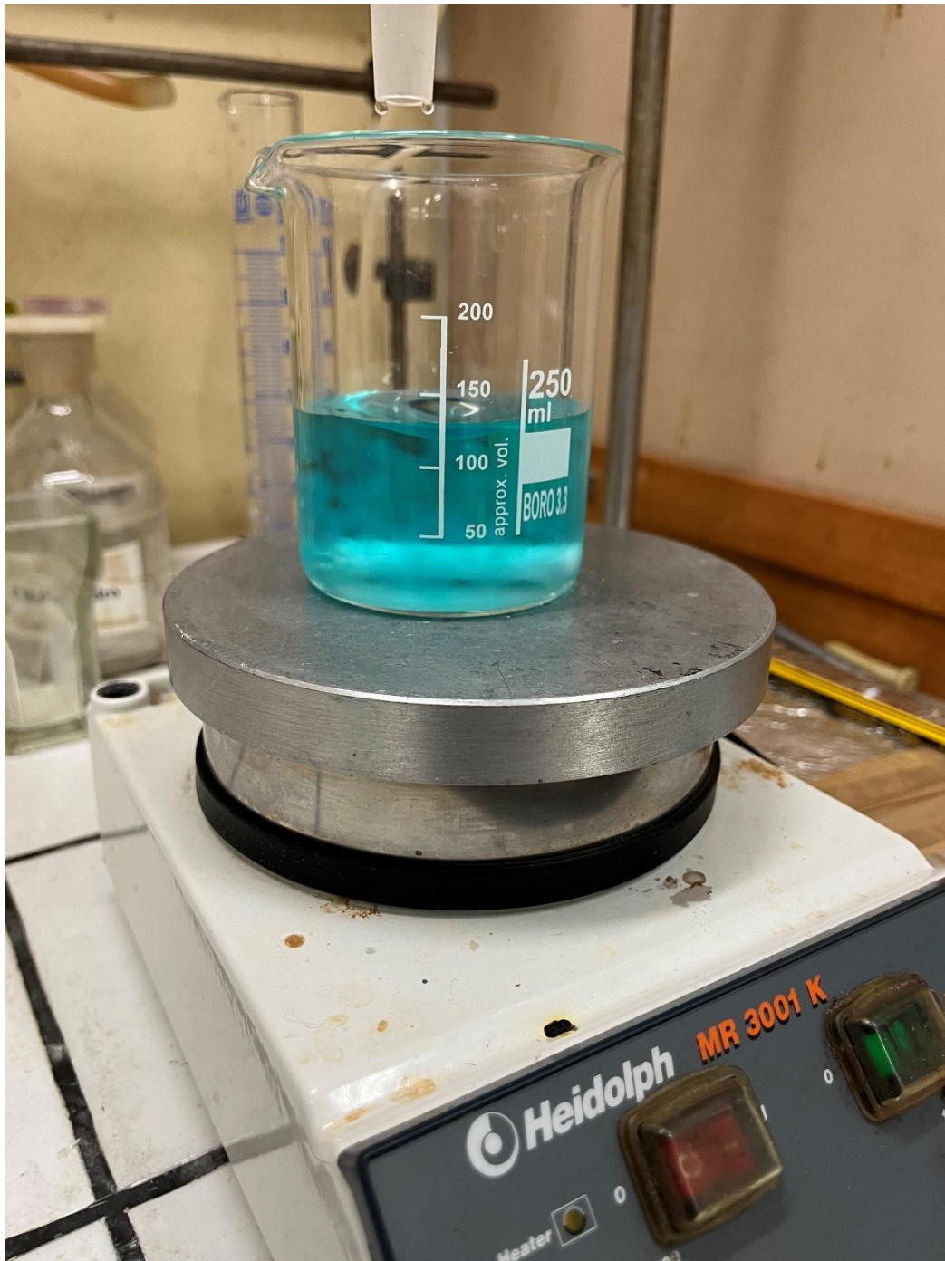
Picture 1. The picture of preparation of Cu-alginate beads from dropping of sodium alginate.
