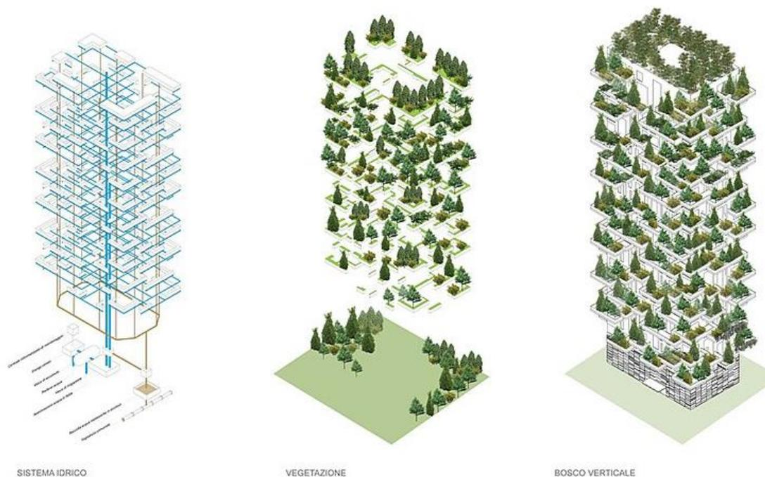
**Figure 32** *The irrigation system of the vegetation in the Bosco Verticale, illustrated in the first figure; Source: Wikipedia*
