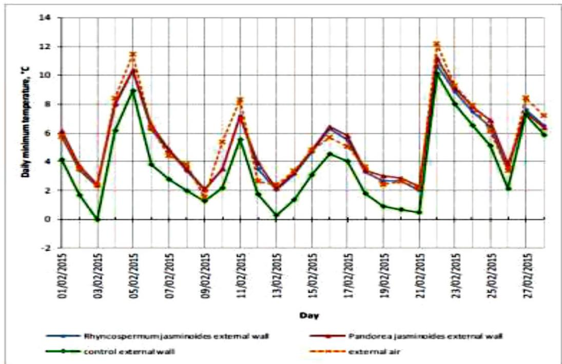
**Figure 29** Daily minimum surface temperature of the external plaster of the three walls exposed to solar radiation and daily maximum external air temperature measured
