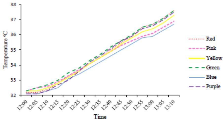
**Figure 52** *Temperature rise of the liquid enclosed in a colored acrylic box*
