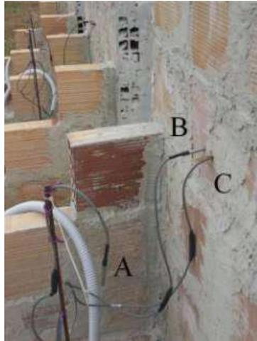
**Figure 28** Location of the temperature sensors: sensor for the indoor temperature inside the volume behind each wall
