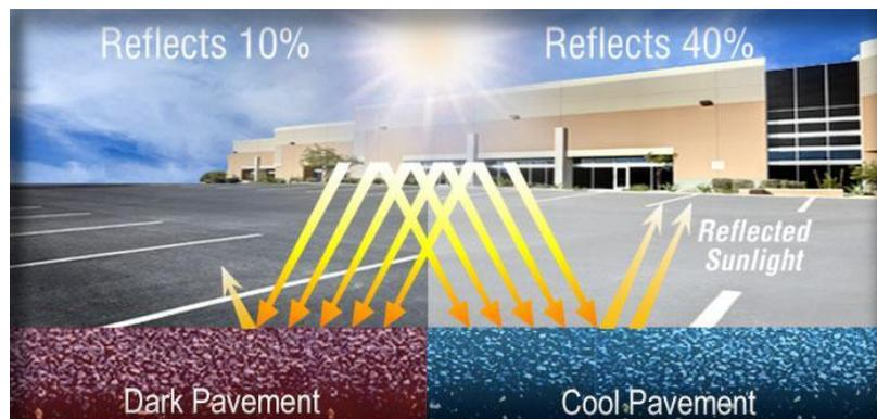
**Figure 5** *Diagram illustrating how Cool Pavement coating will increase solar reflectivity. Source: [www.geographyrealm.com/can-painting-city-streets-reduce-urban-heat-island-effect/](http://www.geographyrealm.com/can-painting-city-streets-reduce-urban-heat-island-effect/)*
