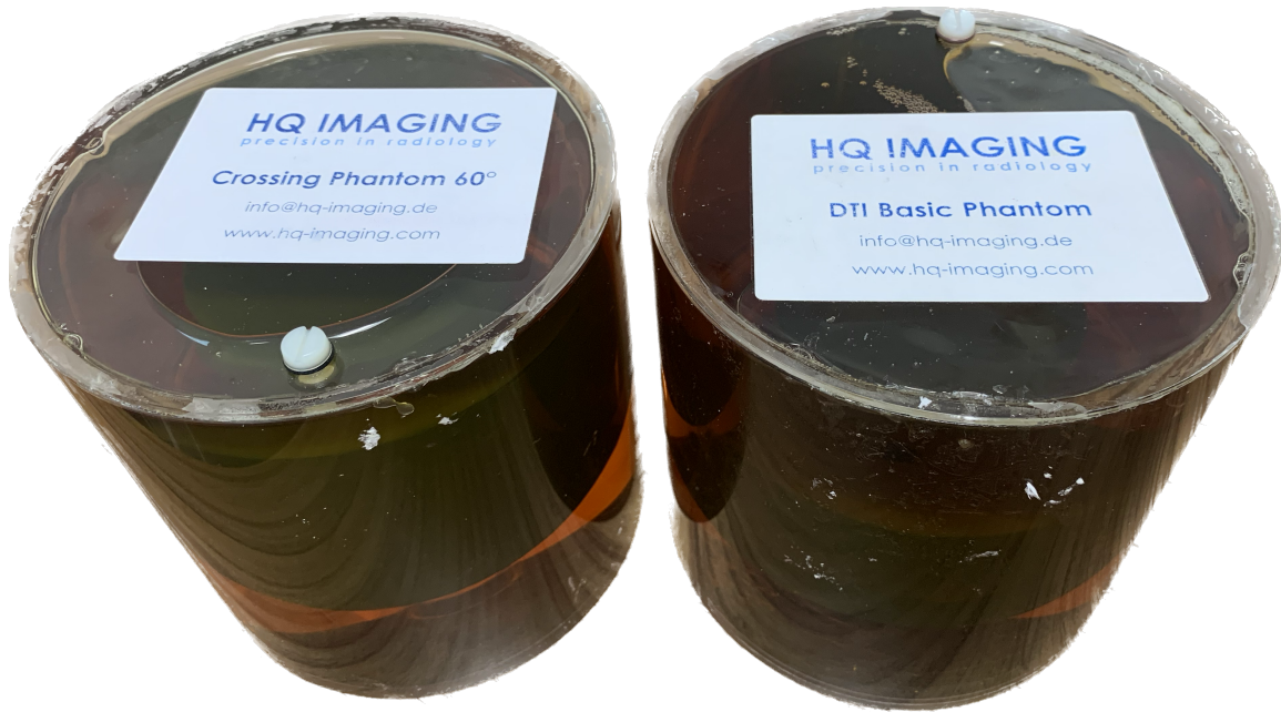
Figure 3.1: Top vision of the DTI phantoms. On the left is shown the crossing phantom, with fibres crossing at 60^\circ , while on the right is shown the basic phantom, with a single fibre ring mimicking restricted anisotropic diffusion.
