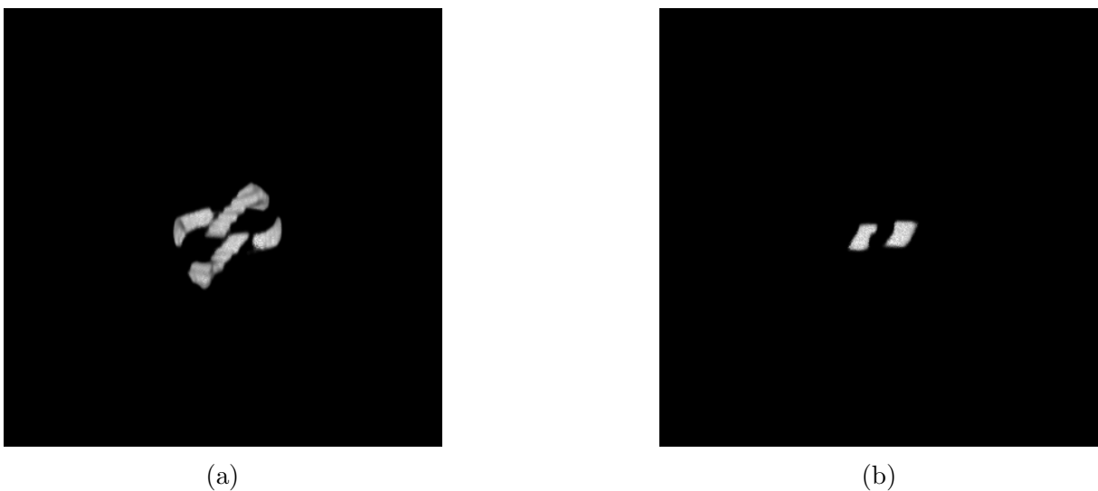
Figure 5.3: Two binary masks were designed to extract diffusion results separately from the rings region and the crossing region of the crossing phantom: (a) mask with only the two rings, and (b) mask for the region where the two fibres cross each other.
