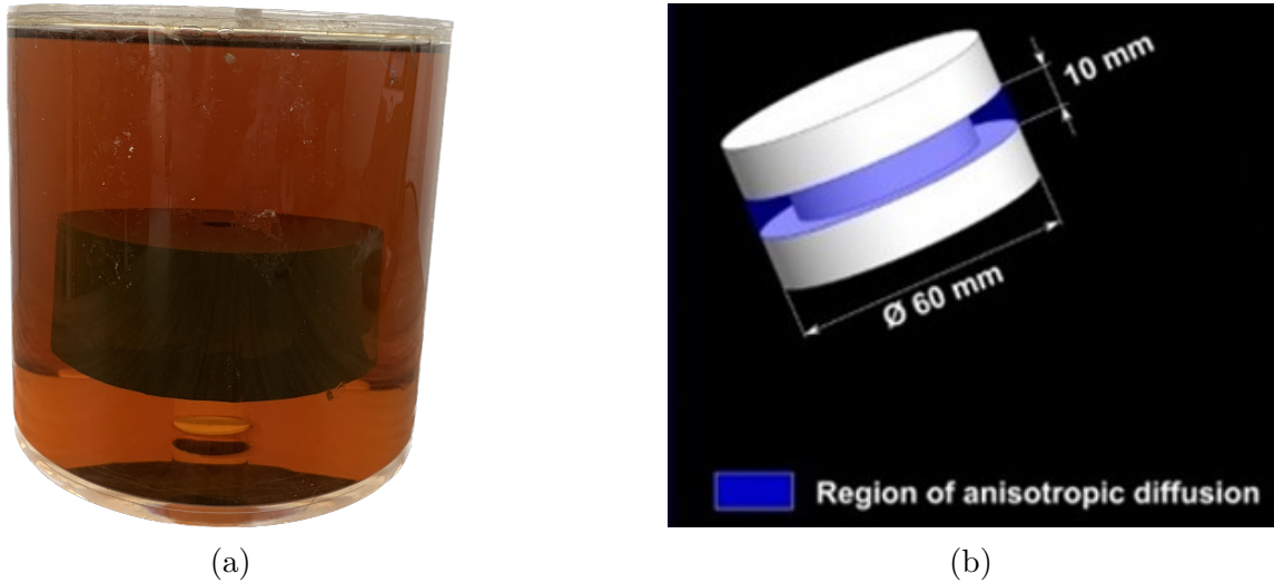
Figure 3.2: (a) Picture of the basic phantom that shows the part in which the fibre bundle is contained and the liquid in which it is immersed. (b) detailed view of the plastic spindle, with the region of anisotropic diffusion highlighted in blue.
