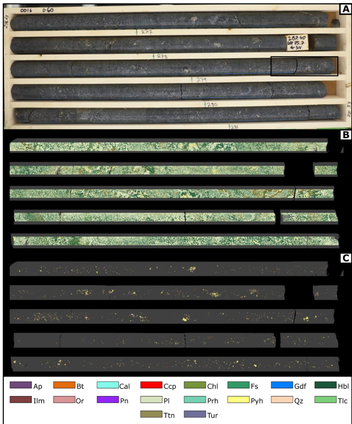
Figure 8 – High-grade zone in KUS0016. A) Core photo with area of detail showed in Figure 9; B) LIBS mineral map; C) LIBS sulfide map.
