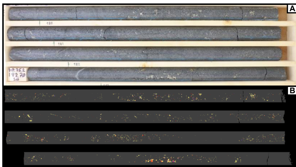
Figure 6 – Disseminated sulfide in vari-textured gabbro from DH0016. A) Core photograph. B) LIBS intermediate resolution core scanning with sulfide mapping image. Yellow: pyrrhotite; purple: pentlandite; red: chalcopyrite.
