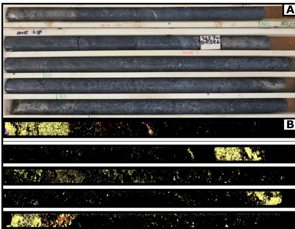
Figure 5 – Semi-massive to disseminated sulfide in vari-textured gabbro from DH0015. A) Core photograph. B) LIBS low resolution core scanning with sulfide mapping image. Yellow: pyrrhotite; purple: pentlandite; red: chalcopyrite.
