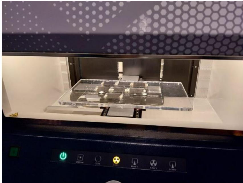
Figure 6: thin sections on the sample holder of \mu -XRF
