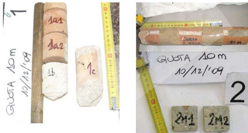
Figure 4-28F: Core samples and cutting mortar layer in standard size for double punch test
