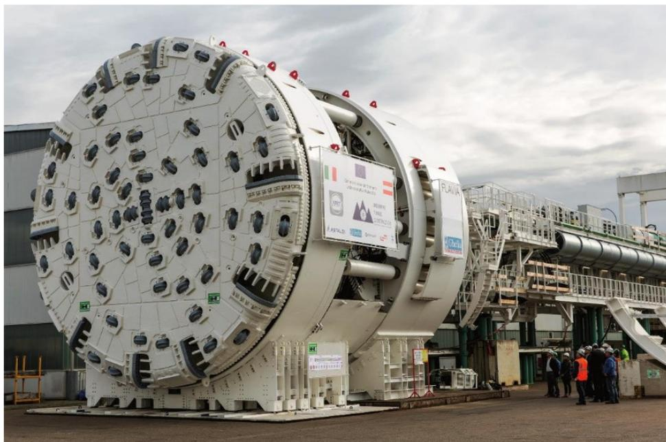
Figura 3. 7 DS-TBM S-1071, TBM “Flavia “. (www.bbt-se.com)
