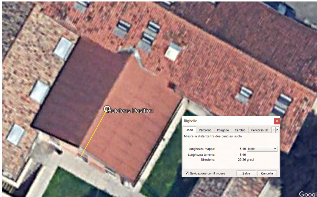
Figure 5.6: HoloLens position determination using Google Earth. By using multiple measures taken by hand inside the laboratory it is possible to measure HoloLens distance with respect to reference points in the map, such as the laboratory walls, thus retrieving the HoloLens position on the map.
