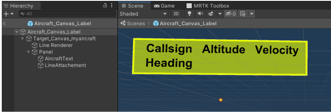
Figure 5.13: Label object visualized in the Unity editor. On the left, in the hierarchy panel, the nested structure of the different elements is visible.
