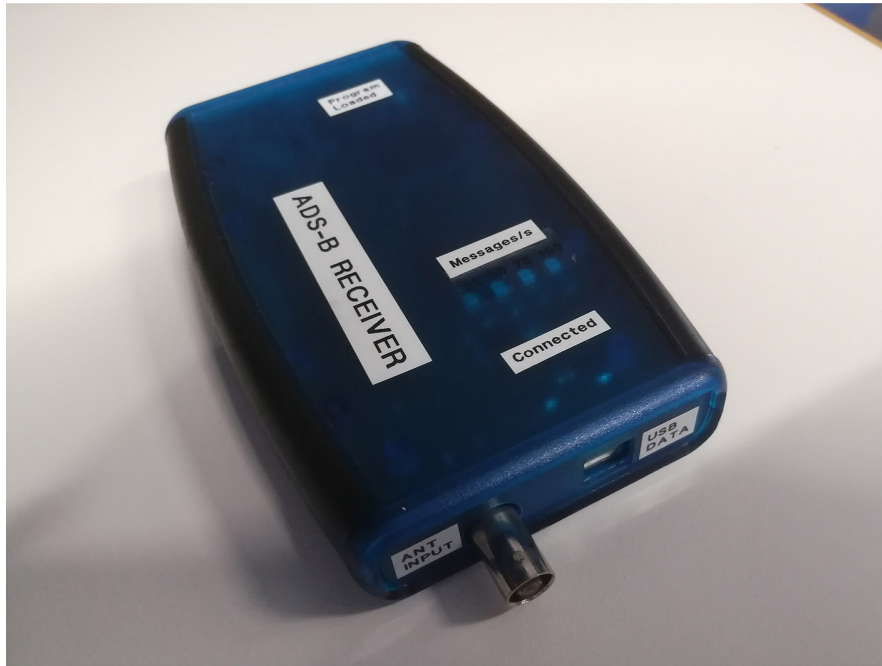
Figure 4.3: ADS-B receiver unit developed by the Systems for InfoMobility Lab.
