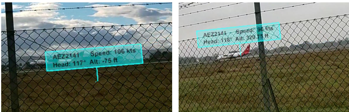
Figure 5.15: Aircraft altitude errors correction. On the left, the aircraft altitude has not been corrected. On the right, the label is well positioned after altitude corrections.
