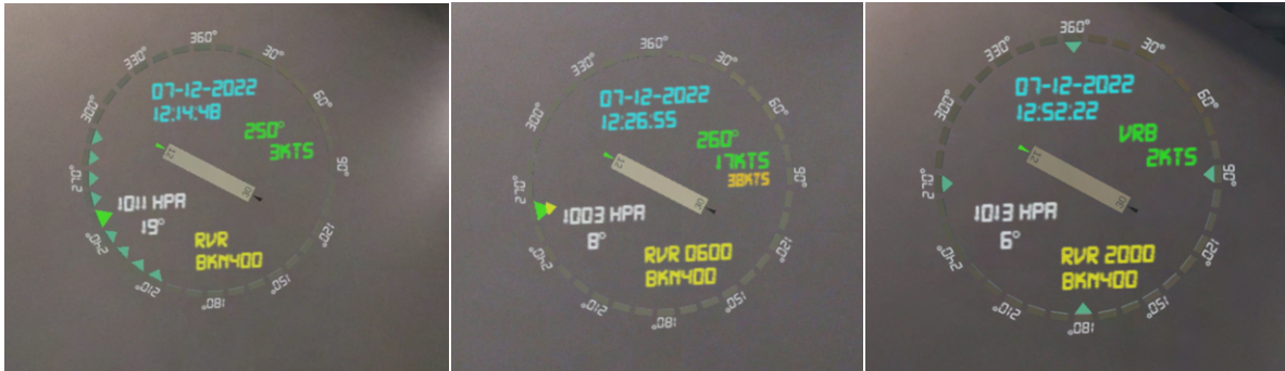
Figure 5.22: METAR visualization examples I. In the first case, the wind is waving as indicated by the smaller green arrows. In the second case, wind gusts are detected (maximum speed 38kts) and are indicated by the yellow arrow. In the third case, the wind has low intensity and variable direction.
