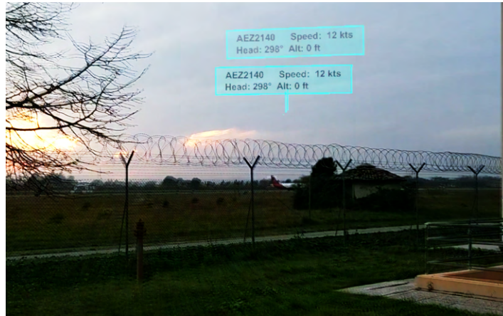
Figure 5.17: Hologram's shaking visualized by merging two consecutive frames of a video recorded on HoloLens while using Camera Canvas rendering.
